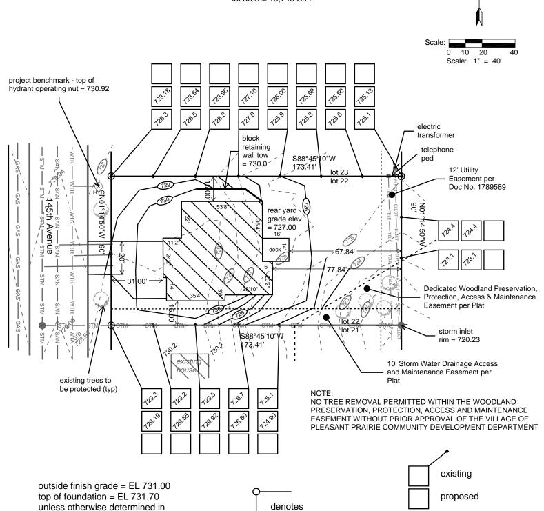
Proposed building field staked true size. Contractor and owner to verify all dimensions before building and adhere to this approved drainage and grading plan. Refer to a current title report for easements or restrictions which may affect the use of this site that are not shown on the recorded subdivision plat.
